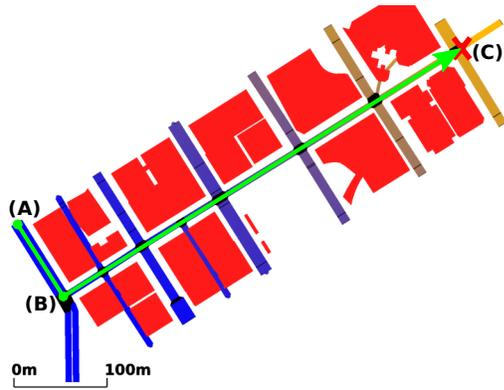
Figure 7. SUMO screenshot showing a 3D road network of downtown Seattle (blue  $\hat{=}$  10 m, orange  $\hat{=}$  65 m, red cross  $\hat{=}$  GLOSA traffic light). The car starts on 1st Avenue at (A), turns on Cherry Street at (B) and continues on to (C).
